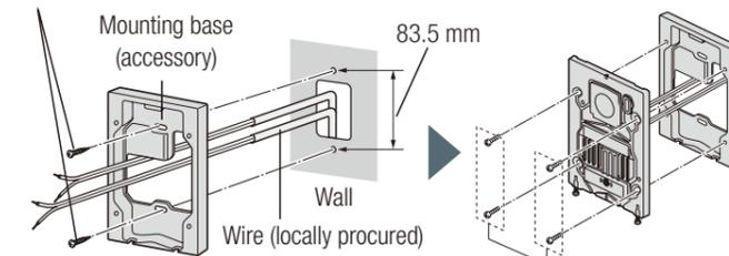
Install the mounting base on a vertical flat wall.
