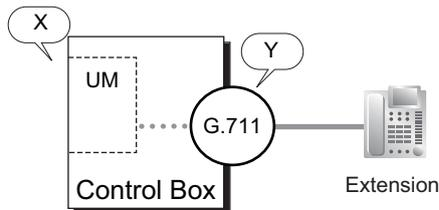
Playing back messages from or recording messages to the Unified Messaging (UM in the figure above) system requires DSP resources, X in this example, in addition to the resources required for the G.711 codec (Y). The total cost is X + Y.
