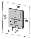
After deciding where to install the main monitor, attach the mounting bracket in the location shown below.
