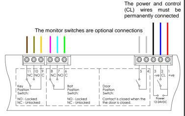
In either fail safe or fail secure configuration, maintained connection of '1' to '2' will keep the DB25K unlocked regardless of door position.
