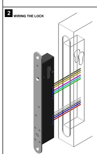
The wiring options and detail is shown overleaf. Once the desired wiring method is chosen run the wires into the rear of the mortice and connect to the lock. There are screw terminals for each wire and a connector guide is shown on the lock cover.
