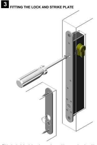
Slide the lock back into the mortice, making sure that the wiring integrity is maintained. Secure the lock and strike plate in place, using the supplied mounting screws. Fit the euro profile cylinder into the lock and secure in place with the M5 screw provided. Ensure that the hole behind the strike plate is free from swarf and is deep enough to allow the lock pin to fully extend when locked.
