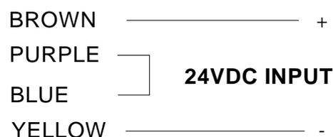
**Warning: Misconnection of wiring will cause the TVS surge suppression inside the electromagnetic lock to fail. This will not be covered under warranty.**
